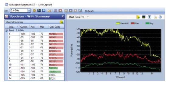
Channels 1, 6 and overlapping channels have a high air time utilisation (duty cycle). The FFT (Fast Fourier Transform) graph shows the interference levels across the band.
