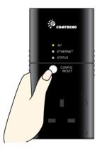
**Step 4:** On the NEW EP adapter you are adding to your network (step 2), press the CONFIG/RESET button until the AP LED starts flashing. The NEW EP adapter AP LED will flash 3 times and the STATUS LED will turn ON.
