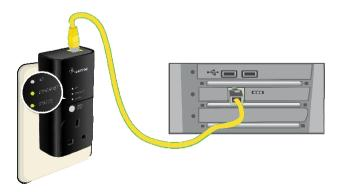
Shortly, you will see the Ethernet LED blinking; this indicates that there is data traffic going through the PG9020. You are now ready to start using your network.
