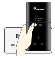
**NOTE:** If you performed a factory reset on the AP adapter (see step 2), it is now an EP adapter. In this case, you will need to assign it as an AP (see FAQ on pg. 8).
