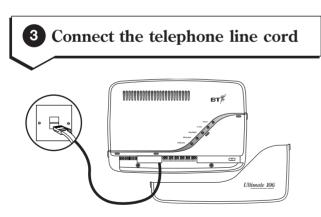
If you do not have modern phone sockets, call **Free***fone 0800* **800 150** and ask for a BT engineer to come and fit the correct type. This is a chargeable service.
