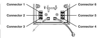
Thread the plastic wire grip through the socket (as shown above).
