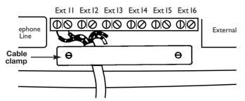
Replace the cable clamp when finished.
