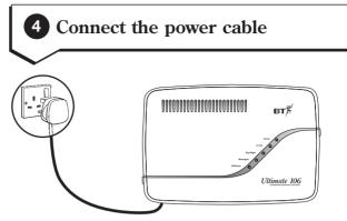
Connect the 3-pin plug into the mains socket and switch the power on. The POWER light comes on.
