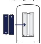
battery cover back into place. markings inside the battery compartment. Then slide the and insert the two batteries supplied. Note the '+' and '-' I Slide off the battery cover from the back of the handset
