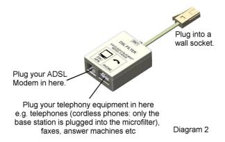
BT ADSL Microfilters are designed to operate in the configuration, as in Diagram 1. Incorrect filters may cause problems with either your telephony products or impede the ADSL speeds.
