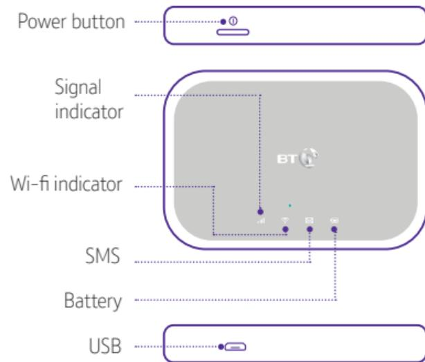
Note: The battery LED will light up when the device is powered on.
