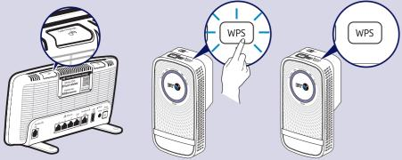
(=) Note: the WPS button on your extender is only used to connect to the router and can't be used to connect devices.
