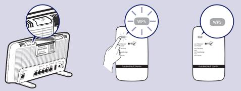
Note: the WPS button on your extender is only used to connect to the router and can't be used to connect devices.
